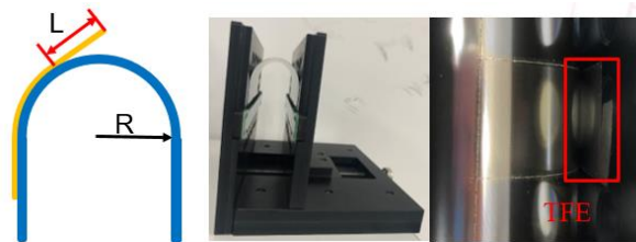
Figure 10. Illustration and equipment for the bending test. Before test, a small region of the TFE is separated from other domains so that the isolated TFE can peel freely.
