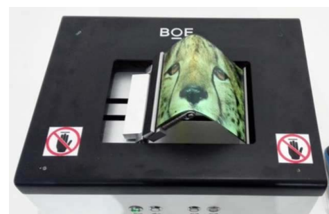
Figure 5. 7.8" flexible OLED display with 5 mm radius bending jig
