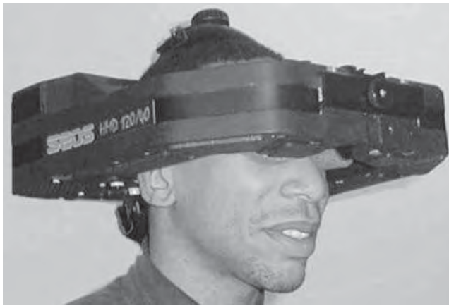
Figure 11.28 Wide-angle field of view HMD. Reprinted courtesy of SOES Displays
