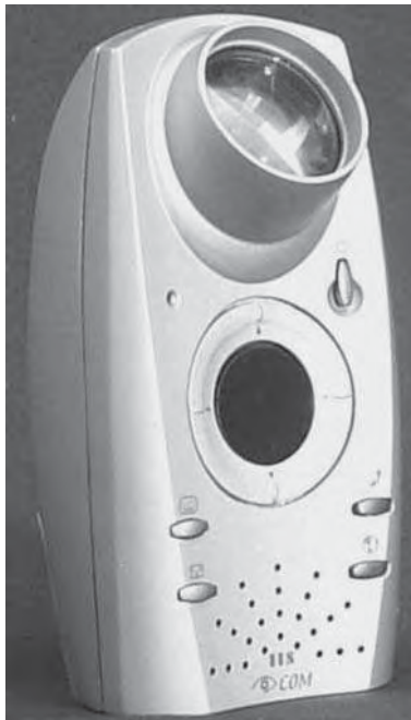
Figure 11.33 Virtual display mounted in prototype hand-held web browser, 4.6 \times 2.5 \times 1.4 inches, weight 6 oz. Reprinted courtesy of Icuity Corp.
