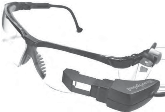
Figure 11.22 Clip-on light pipe relay optics and microdisplay. Reprinted courtesy of MicroOptical Corp.
