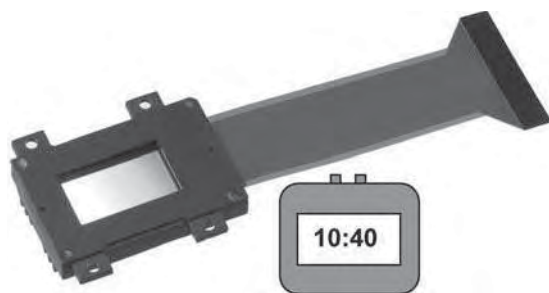
Figure 1.1 Miniature watch display compared with microdisplay having 9\mu\text{m} pixel pitch, 1920 \times 1080 resolution giving active area 0.78-inch diameter. Reprinted courtesy of Sony Corporation
