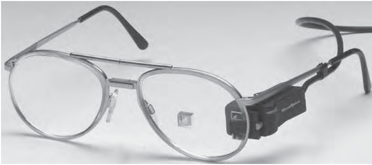
Figure 11.21 Eyeglasses with embedded relay optics and temple mounted microdisplay. Reprinted courtesy of MicroOptical Corp.
