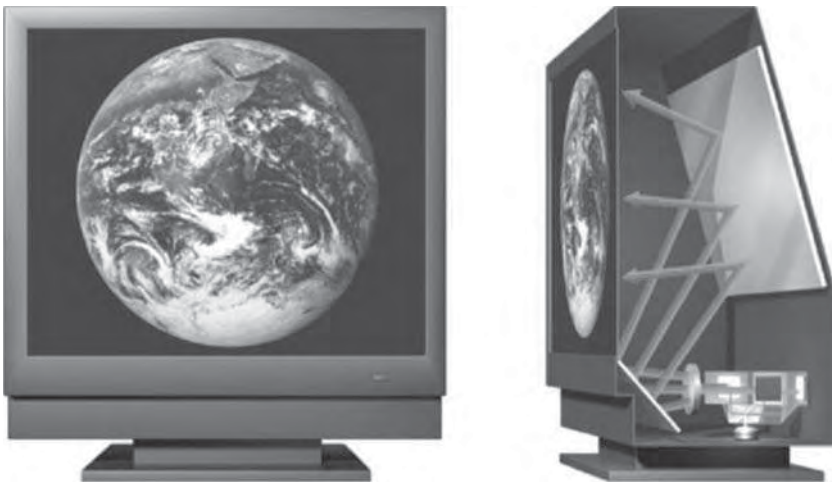
Figure 6.3 Prototype of Syntax-Brilliant's 58-inch rear-projection TV. Reprinted courtesy of Society for Information Display
