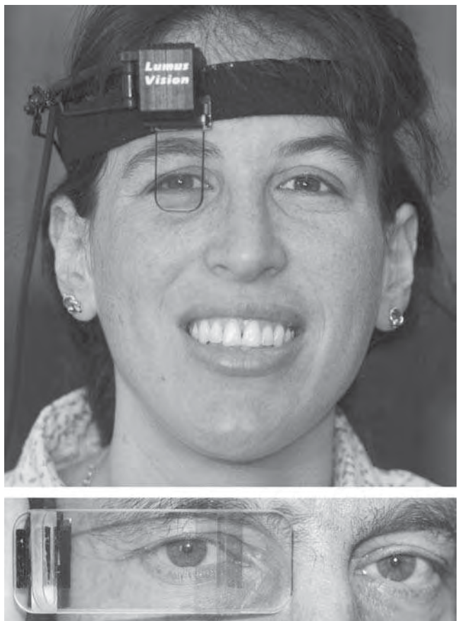
Figure 11.25 LOE near-to-eye display products. Reprinted courtesy of Lumus Ltd
