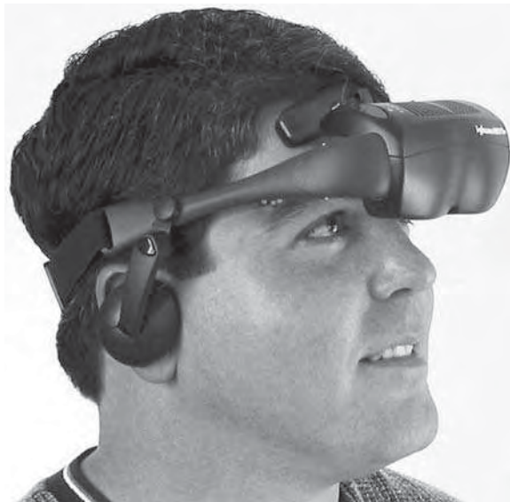
Figure 11.10 SVGA reflective LC microdisplay 3D headset. Reprinted courtesy of i-O Display Systems
